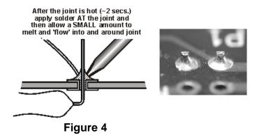
**Figure 6** shows a well-made connection to a single-sided PC board. A small amount of solder has been melted by the heat from the component lead and the PC board pad. A small additional amount of solder has been added to the joint to form a small rising *fillet* around the lead.
