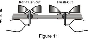
To determine if you are using too much solder, look at your connections once the excess lead length has been trimmed from the component. As shown in **Figures 12 & 13**, if your wire cutters have cut too deeply into the solder, there is probably too much solder being applied.
