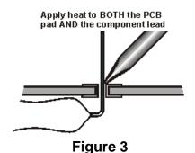
The soldering iron will heat the lead and pad, and their combined heat will then melt the solder. This ensures a well-made, solid joint. (**Figures 4 & 5**)
