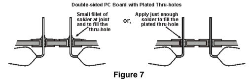
**Note** that some soldering requirements may dictate that *no fillet* be created when soldering to plated-thru holes. (**Figure 7 right**) In this instance, apply only enough solder to *fill* the plated-thru hole. Use of .020" diameter solder greatly enhances your ability to perform this operation. Use of .03" or larger diameter solders will generally cause more solder than required to be applied the instant the solder is applied to the joint.
