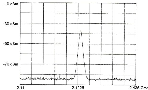
Figure 7: Narrow-band jamming signal used in the jamming tests (2422 MHz).
