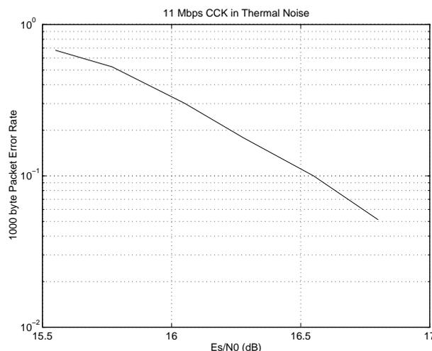
Figure 3: 11 Mbps CCK 1000 byte Packet Error Rate (PER) [5]
