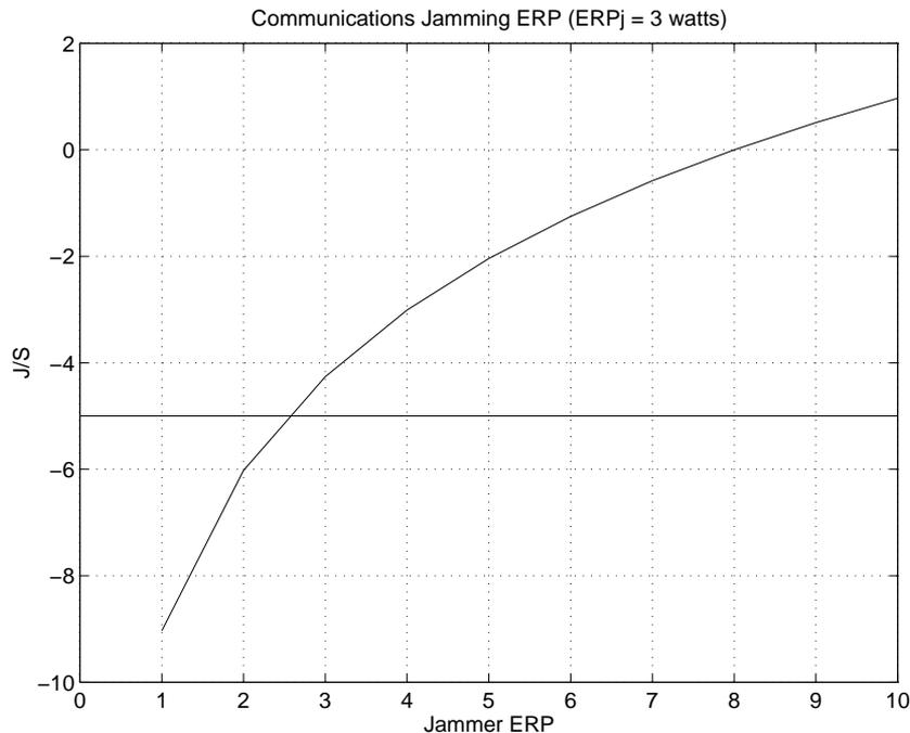
Figure 1: Example of RACH jamming effectiveness calculated using Equation 1. Antenna gain towards both the MS and jammer is supposed to be 12 dBi. Jammer antenna gain is also 12 dBi. MS has a maximum output power of 2 W. Distance from Jammer to BTS is twice the distance between MS and BTS. As the needed J/S for GSM jamming is -5 dB the needed ERP (horizontal axis) can be seen from the graph (2.5 W).
