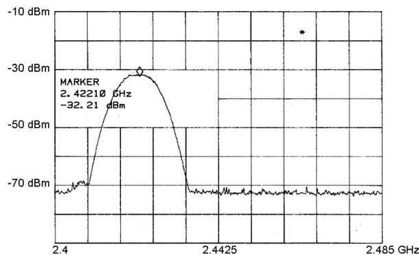
Figure 6: Location of the channel used (number 3) within the 2.4-2.485 GHz ISM band. Notice also the "maximum hold"-shape of the spectrum.
