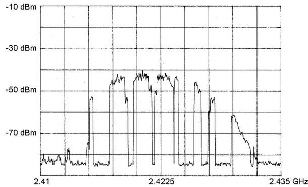
Figure 5: Spectrum of a IEEE 802.11b transmitter measured during the tests.
