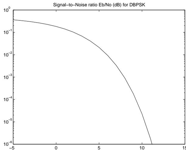
Figure 4: DBPSK bit error probabilities.  $P_e = \frac{1}{2} \exp\left(-\frac{E_b}{N_0}\right)$  [2]
